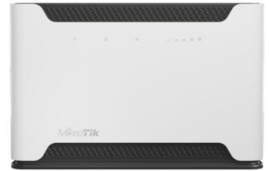
It is a high-speed, dual-band home access point with CAT12 LTE – for really fast Internet anywhere, anytime. But LTE is not the only option – Chateau also features 5 x Gigabit Ethernet ports and a full size USB port.
